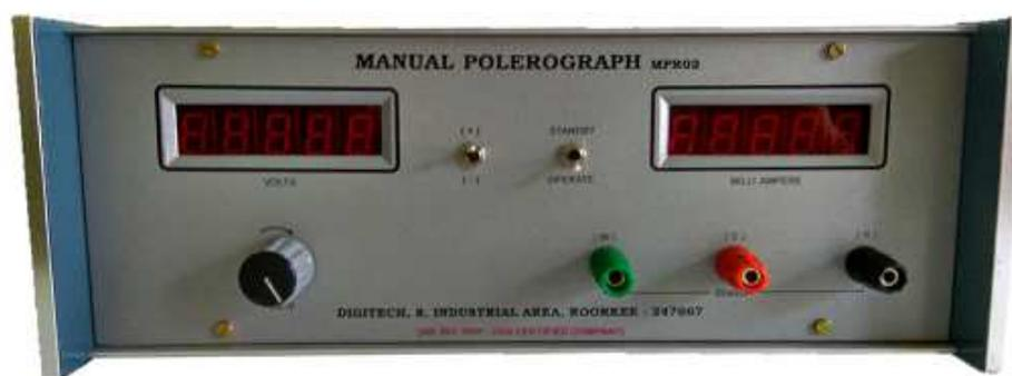
**Manual Polarograph (DG-ME-MP)**, is designed to conduct manual polarography easily and precisely. The potential fed to the electrodes can be continuously varied with adjustable polarity. The reference voltage and the current flow are displayed on digital panel meters. The recorded output is also provided. The unit is mains operated.
